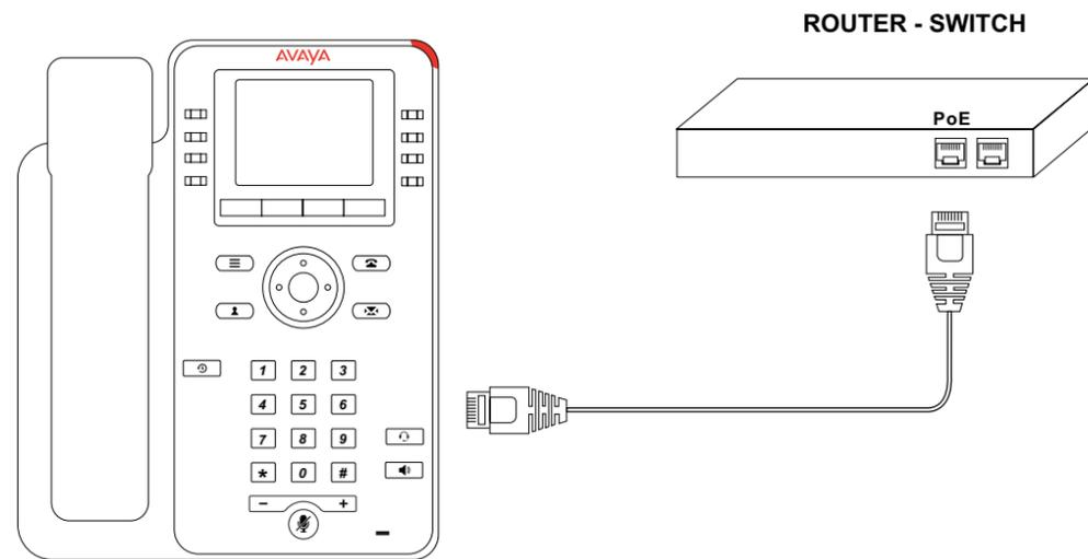
2. If your router does not have PoE port available, connect the J169/J179 ethernet port to the available port on your router. Connect the power adapter to the J169/J179. The device bootup will start.
