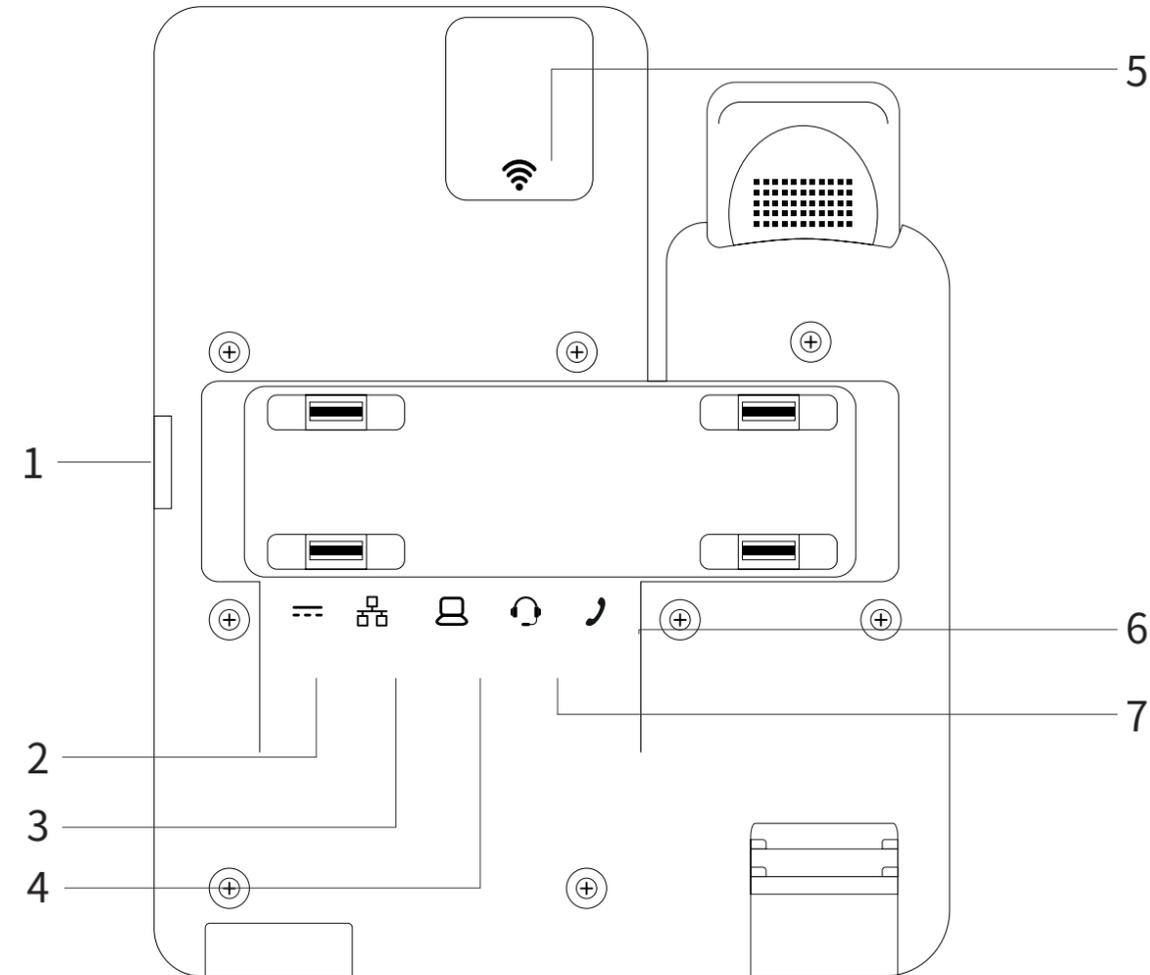
5. **WLAN Module Panel**—To integrate the wireless module for Wi-Fi/Bluetooth support.
